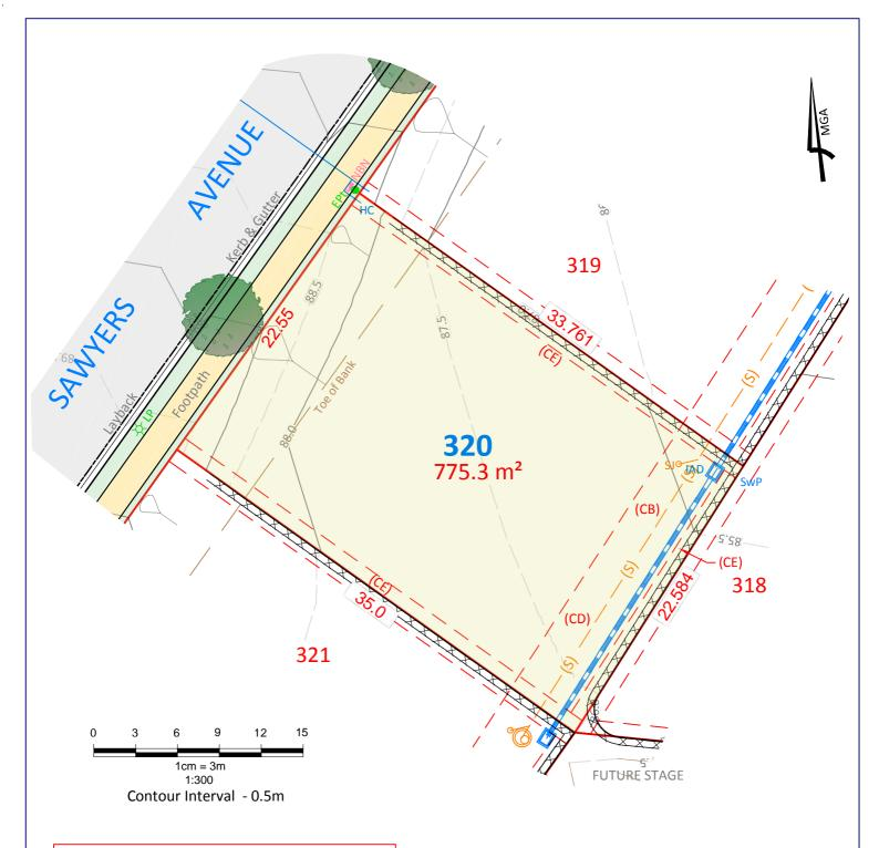
(CB) Easement for sewer gravity main - variable width
