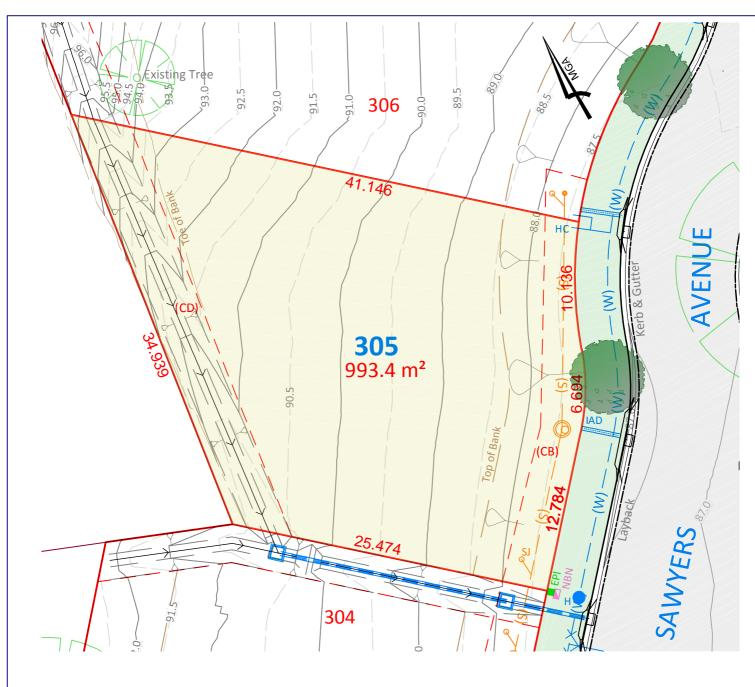
(CB) Easement for sewer gravity main - variable width
