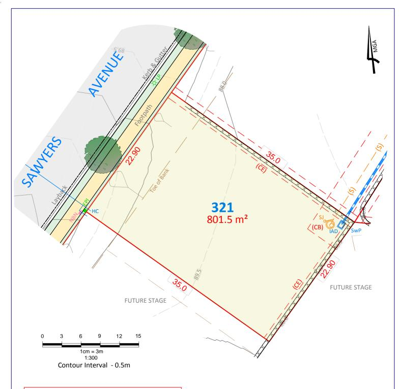
(CB) Easement for sewer gravity main - variable width (CE) Easement for maintenance and repair - 1 wide
