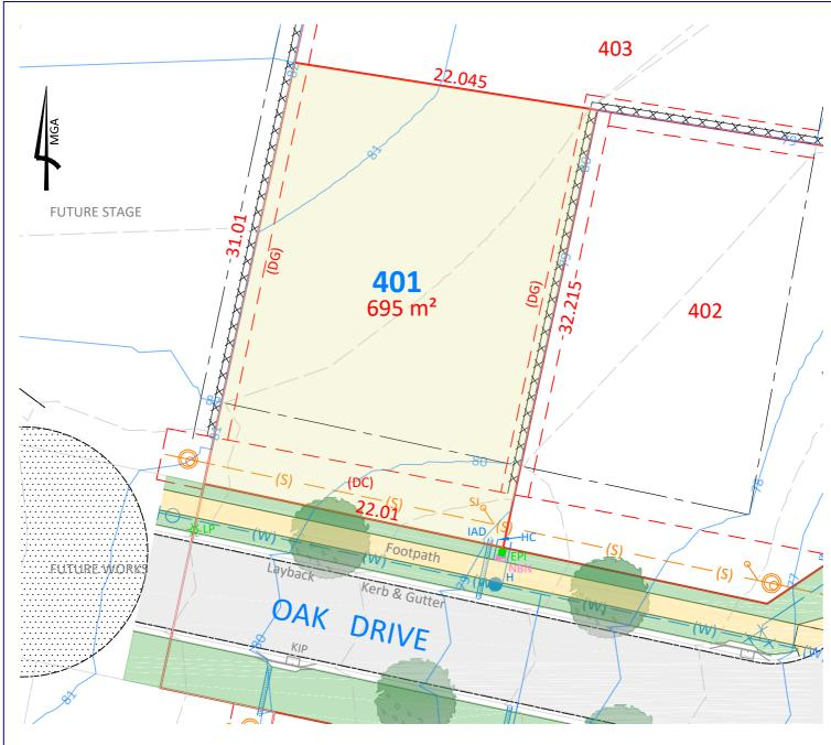
(DC) Easement for sewer gravity main - variable width
