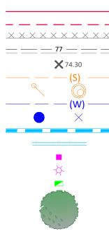
PROPERTY BOUNDARY EASEMENT ROCK RETAINING WALL DESIGN CONTOURS (0.50m INTERVALS) FINISHED SURFACE LEVELS SEWER GRAVITY MAIN SEWER JUNCTION / MANHOLE WATER MAIN (POTABLE) WATER HYDRANT / STOP VALVE STORMWATER DRAINAGE LOT STORMWATER OUTLET ELECTRICAL PILLAR STREET LIGHT NBN PIT
