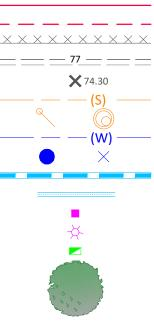
PROPERTY BOUNDARY FASEMENT ROCK RETAINING WALL DESIGN CONTOURS (0.50m INTERVALS) FINISHED SURFACE LEVELS SEWER GRAVITY MAIN SEWER JUNCTION / MANHOLE WATER MAIN (POTABLE) WATER HYDRANT / STOP VALVE STORMWATER DRAINAGE LOT STORMWATER OUTLET ELECTRICAL PILLAR STREET LIGHT NBN PIT
