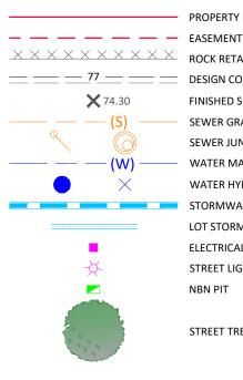
PROPERTY BOUNDARY ROCK RETAINING WALL DESIGN CONTOURS (0.50m INTERVALS) FINISHED SURFACE LEVELS SEWER GRAVITY MAIN SEWER JUNCTION / MANHOLE WATER MAIN (POTABLE) WATER HYDRANT / STOP VALVE STORMWATER DRAINAGE LOT STORMWATER OUTLET ELECTRICAL PILLAR STREET LIGHT NBN PIT
