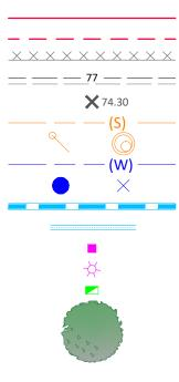
PROPERTY BOUNDARY EASEMENT ROCK RETAINING WALL DESIGN CONTOURS (0.50m INTERVALS) FINISHED SURFACE LEVELS SEWER GRAVITY MAIN SEWER JUNCTION / MANHOLE WATER MAIN (POTABLE) WATER HYDRANT / STOP VALVE STORMWATER DRAINAGE LOT STORMWATER OUTLET ELECTRICAL PILLAR STREET LIGHT NBN PIT
