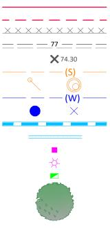
PROPERTY BOUNDARY EASEMENT ROCK RETAINING WALL DESIGN CONTOURS (0.50m INTERVALS) FINISHED SURFACE LEVELS SEWER GRAVITY MAIN SEWER JUNCTION / MANHOLE WATER MAIN (POTABLE) WATER HYDRANT / STOP VALVE STORMWATER DRAINAGE LOT STORMWATER OUTLET ELECTRICAL PILLAR STREET LIGHT NBN PIT STREET TREE
